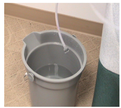
Place Chemical Feed Hose into Rinse Solution
